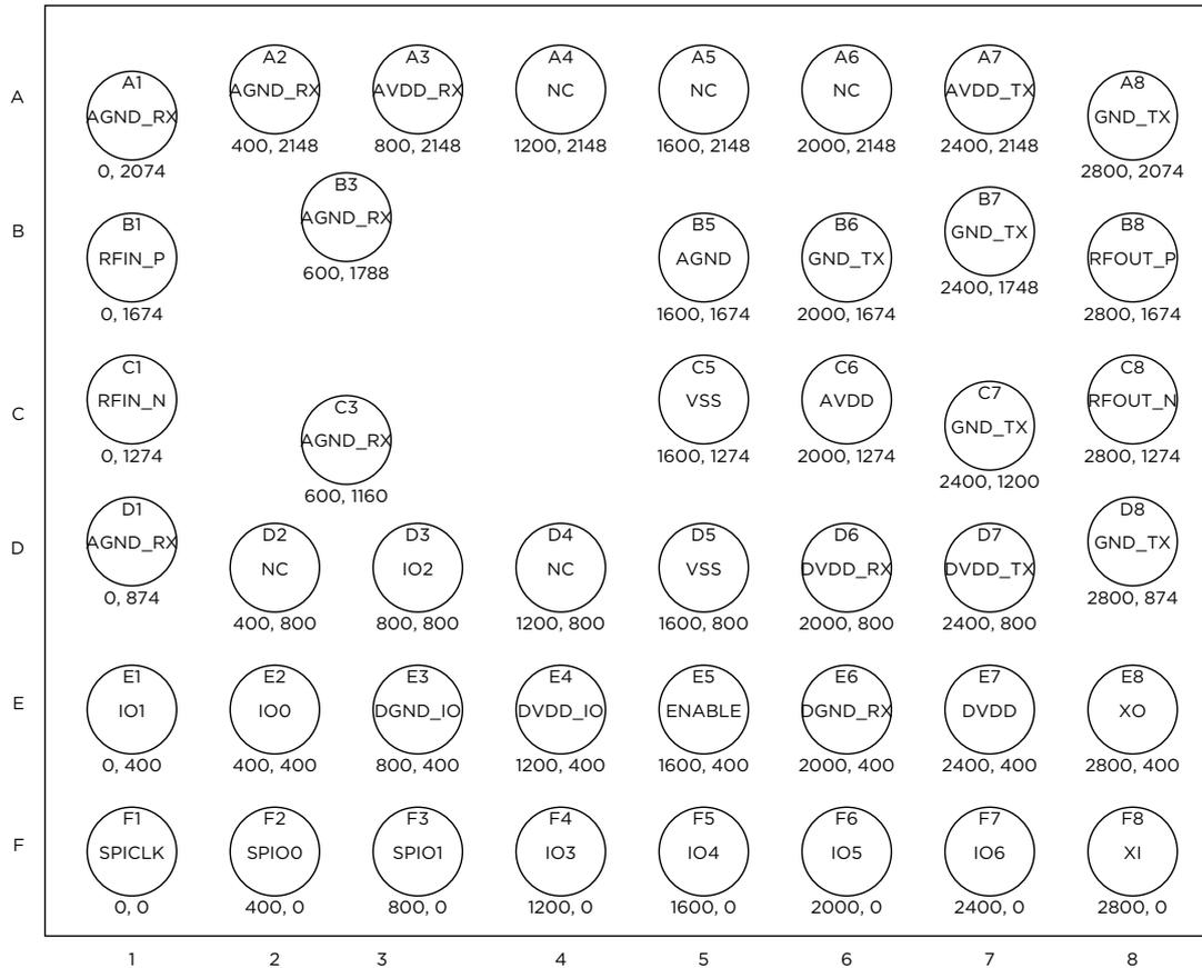
Figure 2.1. Top view footprint (coordinates in micrometers)
